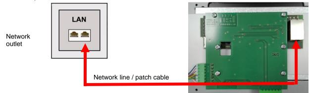
After the WATERFRIEND was connected to an active network outlet, the power supply can be turned on. The web server in WATERFRIEND now searches autonomously for the communication server and logs on to the database.
