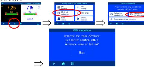
The ORP electrode is immersed in the 468mV buffer solution. The current value for the ORP electrode is then shown in the display. The discrepancy between the displayed value and the buffer solution value (468mV) should not exceed  $\pm$  10%. If there is a large discrepancy or extended reaction time, the electrode should be replaced as soon as possible.
