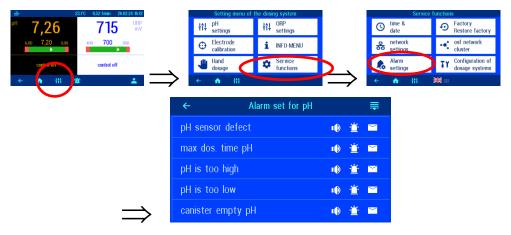
For each individual alarm type, you can choose whether an acoustic alarm is generated ( $\langle \square \rangle$ ), an e-mail is sent ( $\boxtimes$ ), or the collective fault message is activated ( $\boxtimes$ ).
