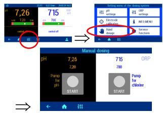
Each metering pump can be switched on and off individually by pressing the appropriate keys. While doing so, please observe the corresponding status display. The maximum runtime is limited to 60 seconds. Once this time has elapsed, the pumps will be switched off automatically. The remaining runtime is shown graphically in the display.
