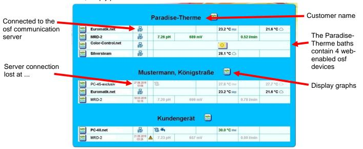
In order to use the communication server, the option "Internet connection via communication server" must be enabled in the control unit itself (default factory setting):
