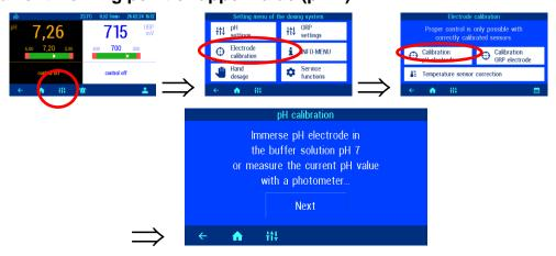
If the calibration is to be carried out using a photometer during operation as a one-point calibration, the actual pH value of the pool water should now be determined using a photometer. If the calibration is to be carried out using buffer solutions, the pH electrode must be unscrewed from the flow fitting and then immersed in the green "pH 7" buffer solution.
