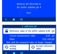
During calibration, the slope of the electrode is shown on the display. The slope must be in a range between 45.0 to 65.0 mV. Otherwise, the message "Large deviation" appears on the display.
