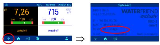
After you have entered the device ID in your user profile, your device will appear in your device overview and can be operated using the communication server:
