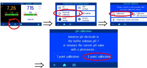
At the "professional level" a two-point calibration of the pH sensor is also possible.
